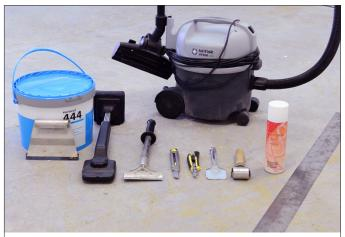
First make sure the following is available: Carpet glue and trowel a knee kicker a floor scraper a utility knife a hooked knife an appropriate metal bolster a metal roller anti-fraying spray a short ruler (max 1 meter)
